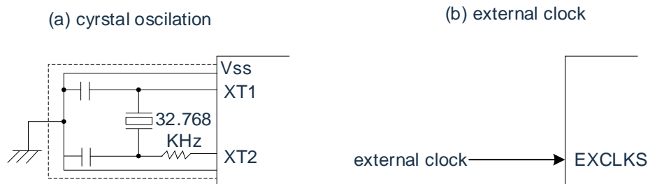
Figure4-13 Example of External Circuit of XT1 Oscillation Circuit
